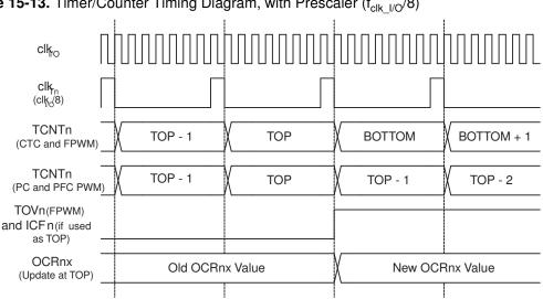
Figure 15-13. Timer/Counter Timing Diagram, with Prescaler ( $f_{clk}$  I/O/8)
