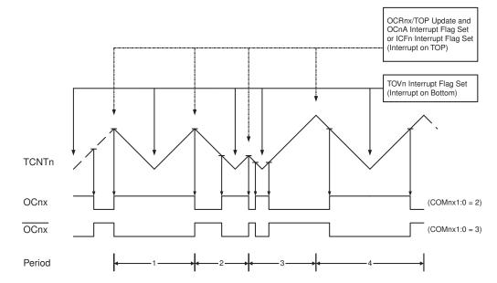
Figure 15-8. Phase Correct PWM Mode, Timing Diagram
