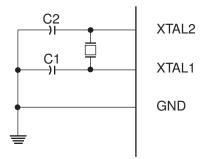
The Oscillator can operate in three different modes, each optimized for a specific frequency range. The operating mode is selected by the fuses CKSEL3..1 as shown in Table 4.
