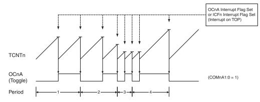
Figure 15-6. CTC Mode, Timing Diagram
