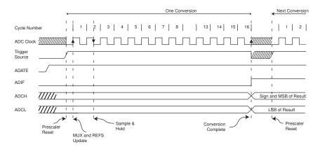
Figure 21-6. ADC Timing Diagram, Auto Triggered Conversion
