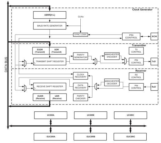
The EUSART is activated with the EUSART bit of EUCSRB register. Until this bit is not set, the USART will behave as standard USART, all the functionnalities of the EUSART are not accessible.
