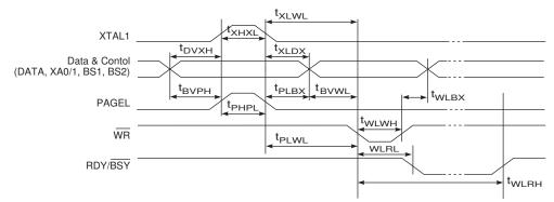
Figure 25-8. Parallel Programming Timing, Loading Sequence with Timing Requirements<sup>(1)</sup>
