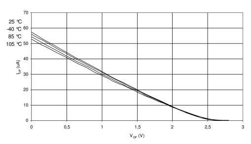
Figure 27-15. Reset Pull-Up Resistor Current vs. Reset Pin Voltage ( $V_{CC}$  = 2.7V) PE0 and RESET PULL-UP RESISTOR CURRENT vs. INPUT VOLTAGE Vcc = 2.7 V
