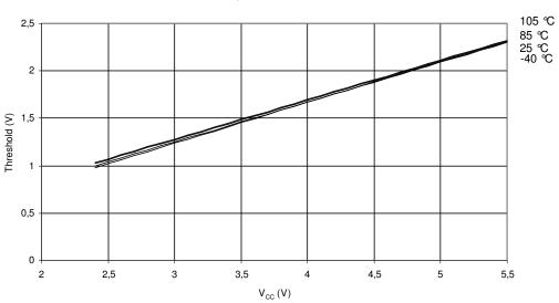
Figure 27-23. Reset Input Threshold Voltage vs. V<sub>CC</sub> (VIL, Reset Pin Read As '0') RESET INPUT THRESHOLD VOLTAGE vs. V<sub>CC</sub> VIL, RESET PIN READ AS '0'
