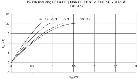
Figure 27-19. I/O Pin Sink Current vs. Output Voltage (V<sub>CC</sub> = 2.7V) I/O PIN (including PE1 & PE2) SINK CURRENT vs. OUTPUT VOLTAGE Vcc = 2.7 V
