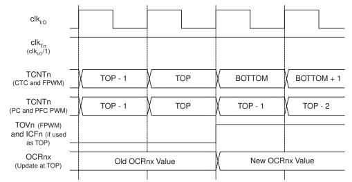
Figure 15-12. Timer/Counter Timing Diagram, no Prescaling
