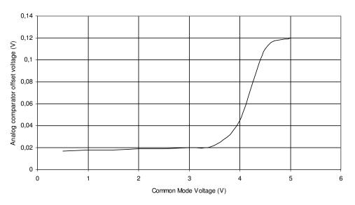
Note: corrected on AT90PWM216/316 to allow almost full scale use.
