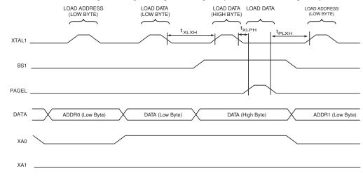
Note: 1. The timing requirements shown in Figure 25-7 (i.e., t<sub>DVXH</sub>, t<sub>XHXL</sub>, and t<sub>XLDX</sub>) also apply to loading operation.
