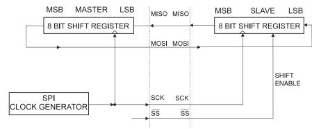
Figure 17-2. SPI Master-slave Interconnection
