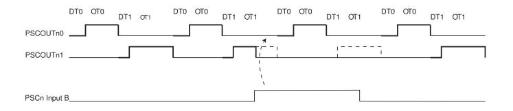
The output is disactivated while retriggering input is active.
