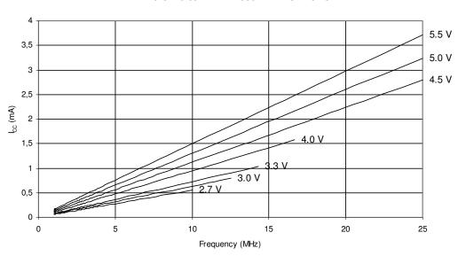
RESET SUPPLY CURRENT vs.  $V_{CC}$  excluding current through the reset pullup
