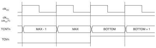
Figure 14-8. Timer/Counter Timing Diagram, no Prescaling
