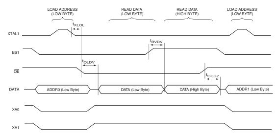
Note: 1. ggThe timing requirements shown in Figure 26-5 (i.e., t<sub>DVXH</sub>, t<sub>XHXL</sub>, and t<sub>XLDX</sub>) also apply to reading operation.
