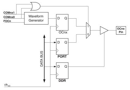
The general I/O port function is overridden by the Output Compare (OC0x) from the Waveform Generator if either of the COM0x1:0 bits are set. However, the OC0x pin direction (input or output) is still controlled by the Data Direction Register (DDR) for the port pin. The Data Direction Register bit for the OC0x pin (DDR\_OC0x) must be set as output before the OC0x value is visible on the pin. The port override function is independent of the Waveform Generation mode.
