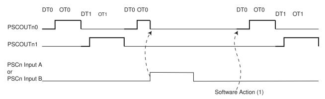
Note: 1. Software action is the setting of the PRUNn bit in PCTLn register.
