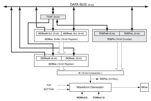
Figure 15-4. Output Compare Unit, Block Diagram
