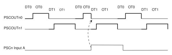
Figure 16-31. PSC behaviour versus PSCn Input A in Mode 8
