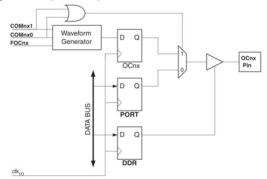
Figure 15-5. Compare Match Output Unit, Schematic
