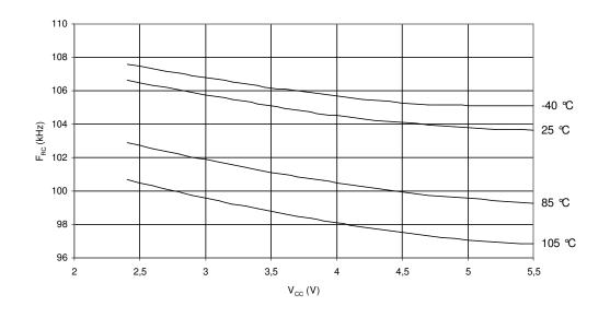
Figure 27-35. Watchdog Oscillator Frequency vs. V<sub>CC</sub> WATCHDOG OSCILLATOR FREQUENCY vs. OPERATING VOLTAGE
