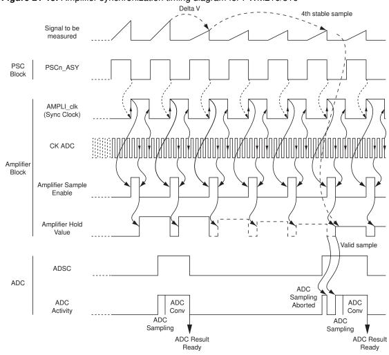
Figure 21-15. Amplifier synchronization timing diagram for PWM216/316
