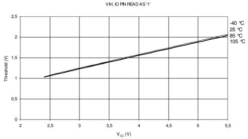
Figure 27-20. I/O Pin Input Threshold Voltage vs. V<sub>CC</sub> (VIH, I/O Pin Read As '1') I/O PIN (including PE1 & PE2) INPUT THRESHOLD VOLTAGE vs.  $V_{\mbox{\tiny CC}}$
