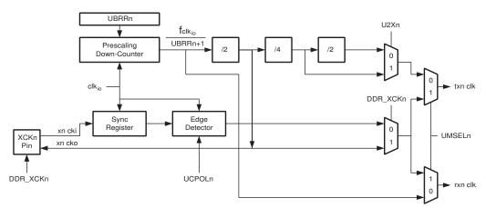
Figure 18-2. USART Clock Generation Logic, Block Diagram
