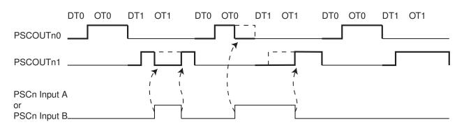
Figure 16-26. PSC behaviour versus PSCn Input A or Input B in Mode 4
