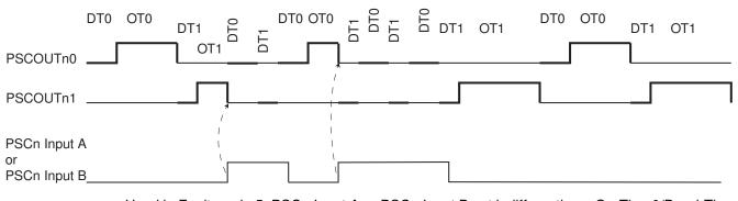
Used in Fault mode 5, PSCn Input A or PSCn Input B act indifferently on On-Time0/Dead-Time0 or on On-Time1/Dead-Time1.
