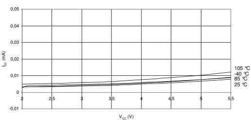
RESET CURRENT vs.  $V_{\text{CC}}$  (CLOCK STOPPED) EXCLUDING CURRENT THROUGH THE RESET PULLUP
