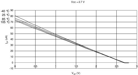
I/O PIN (including PE1 & PE2) PULL-UP RESISTOR CURRENT vs. INPUT VOLTAGE
