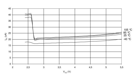
BROWNOUT DETECTOR CURRENT vs. V<sub>CC</sub>
