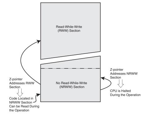
Figure 24-1. Read-While-Write vs. No Read-While-Write
