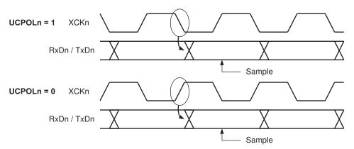
The UCPOL bit UCRSnC selects which XCK clock edge is used for data sampling and which is used for data change. As Figure 18-3 shows, when UCPOL is zero the data will be changed at rising XCK edge and sampled at falling XCK edge. If UCPOL is set, the data will be changed at falling XCK edge and sampled at rising XCK edge.
