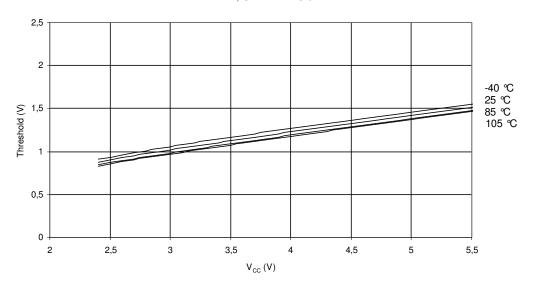
Figure 27-22. Reset Input Threshold Voltage vs. V<sub>CC</sub> (VIH, Reset Pin Read As '1') RESET INPUT THRESHOLD VOLTAGE vs. V<sub>CC</sub> VIH, RESET PIN READ AS '1'
