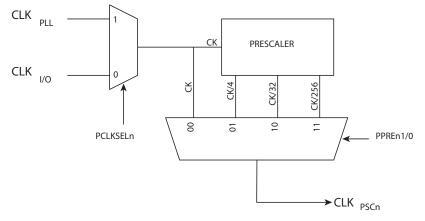
PCLKSELn bit in PSC n Configuration register (PCNFn) is used to select the clock source.
