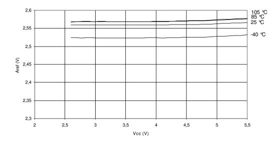
Figure 27-34. AREF Voltage vs. Temperature AREF VOLTAGE vs. TEMPERATURE
