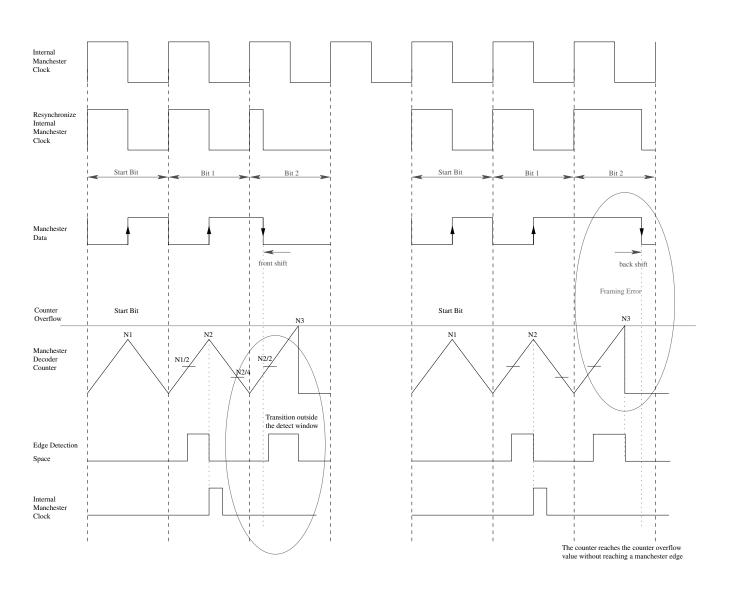
Figure 19-5. Manchester Frame error detection
