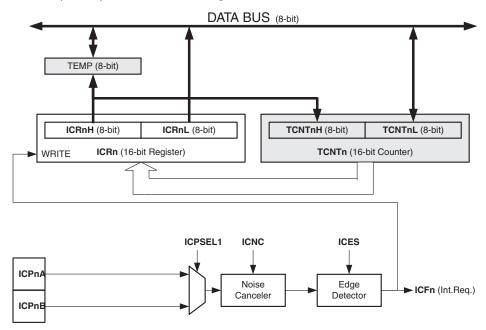
Figure 15-3. Input Capture Unit Block Diagram
