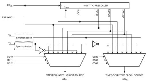
Figure 13-2. Prescaler for Timer/Counter0 and Timer/Counter1<sup>(1)</sup>
