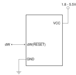
Figure 23-1. The debugWIRE Setup
