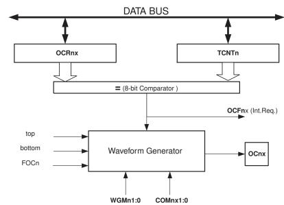
Figure 14-3. Output Compare Unit, Block Diagram
