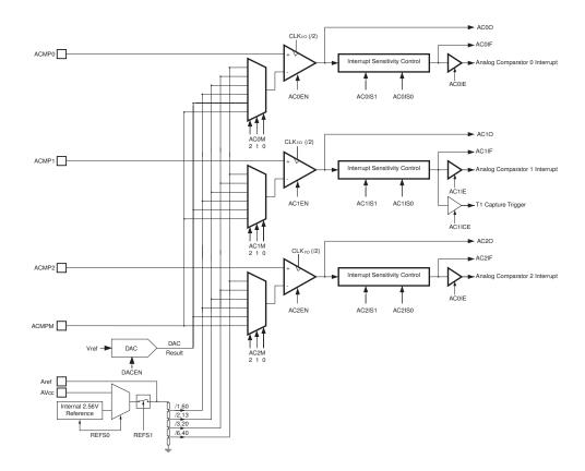
Figure 20-1. Analog Comparator Block Diagram<sup>(1)(2)</sup>
