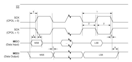
Figure 26-3. SPI Interface Timing Requirements (Master Mode)
