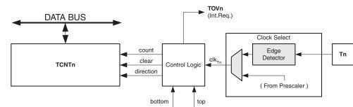
Figure 14-2. Counter Unit Block Diagram
