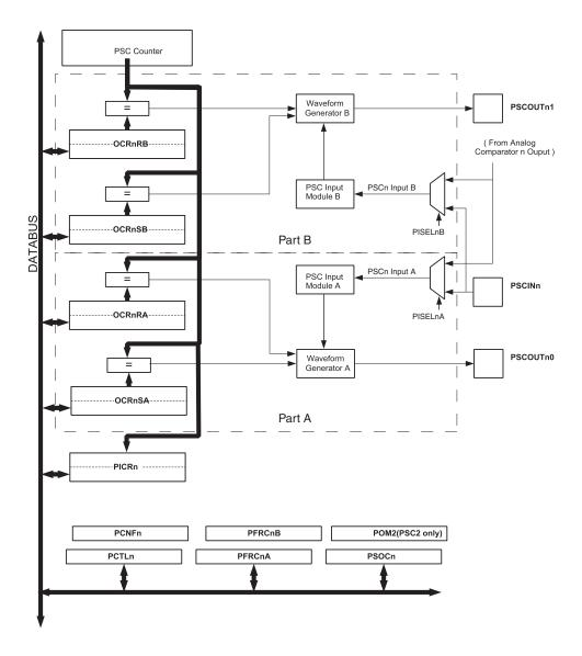
Figure 16-1. Power Stage Controller 0 or 1 Block Diagram
