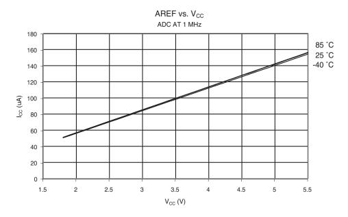
Figure 27-42. Analog Comparator Current vs.  $V_{CC}$  ANALOG COMPARATOR CURRENT vs.  $V_{CC}$
