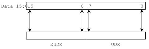
For 17 bit character the seventeenth bit is locate in RxB8 or TXB8 register. In transmitter mode, the data should be written MSB first. The data transmission starts when the UDR register is written.
