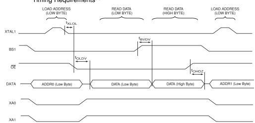
**Figure 25-9.** Parallel Programming Timing, Reading Sequence (within the Same Page) with Timing Requirements<sup>(1)</sup>
