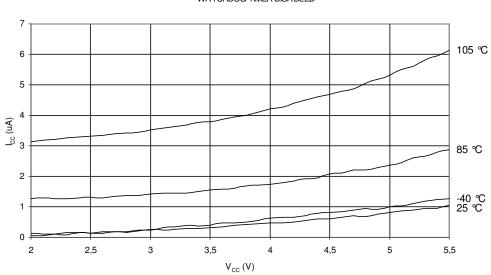
Figure 27-9. Power-Down Supply Current vs. V<sub>CC</sub> (Watchdog Timer Disabled) POWER-DOWN SUPPLY CURRENT vs. V<sub>CC</sub> WATCHDOG TIMER DISABLED
