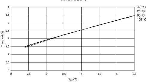
Figure 27-27. PE0 Input Threshold Voltage vs. V<sub>CC</sub> (PE0 Pin Read As '1') PE0 INPUT THRESHOLD VOLTAGE vs. V<sub>CC</sub> VIH, PE0 PIN READ AS '1'
