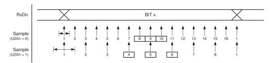
Figure 18-7. Sampling of Data and Parity Bit
