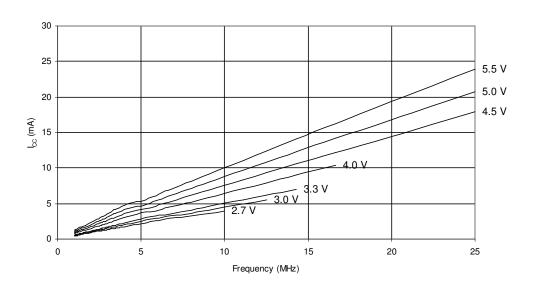
Figure 27-3. Active Supply Current vs. V<sub>CC</sub> (Internal RC Oscillator, 8 MHz)
