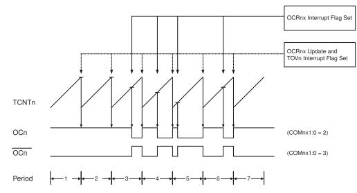
Figure 14-6. Fast PWM Mode, Timing Diagram
