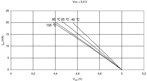
I/O PIN (including PE1 & PE2) SOURCE CURRENT vs. OUTPUT VOLTAGE Vcc = 5.0 V
