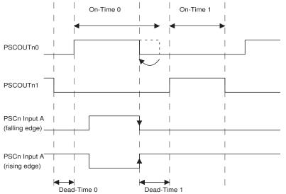
Note: This exemple is given in "Input Mode 8" in "2 or 4 ramp mode" See Figure 16-31. for details.
