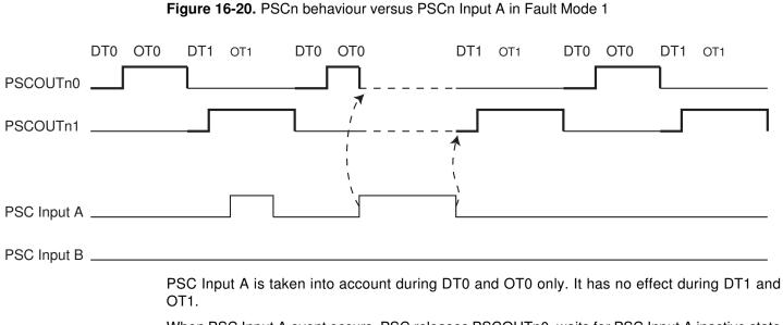
When PSC Input A event occurs, PSC releases PSCOUTn0, waits for PSC Input A inactive state and then jumps and executes DT1 plus OT1.
