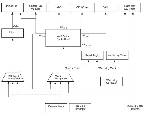
Figure 7-1. Clock Distribution AT90PWM216/316
