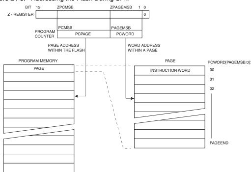
**Figure 24-3.** Addressing the Flash During SPM<sup>(1)</sup>
