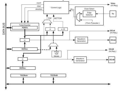
Figure 14-1. 8-bit Timer/Counter Block Diagram
